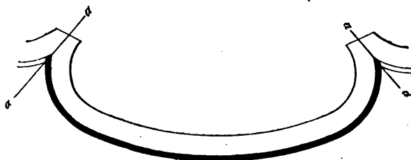
Fig. 61.—Diagram Showing Method of Purfling Waists and Cutting Mitres.
